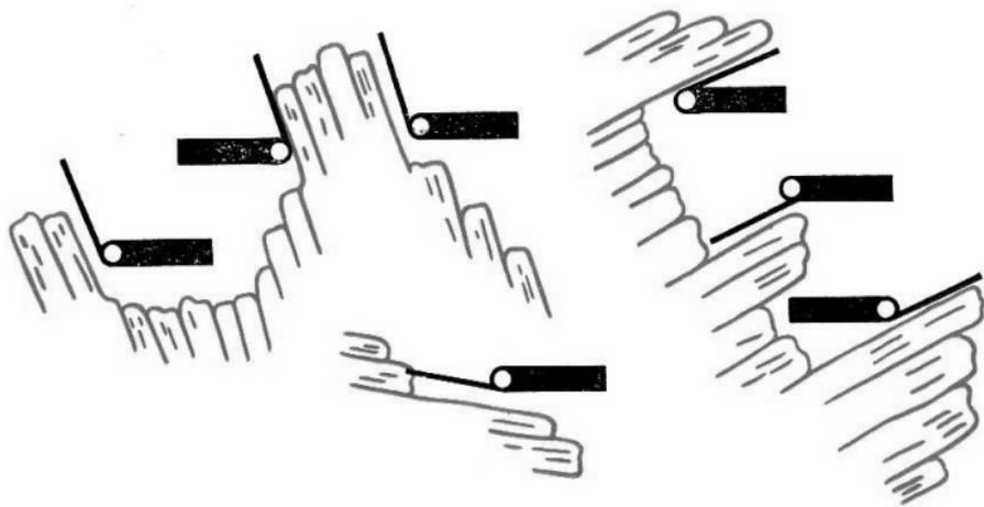
Fig. 4 Backing the inclination measuring plate against the downthrow side
