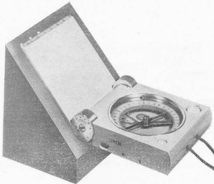
Fig. 5 Backing the inclination measuring plate against the hanging
